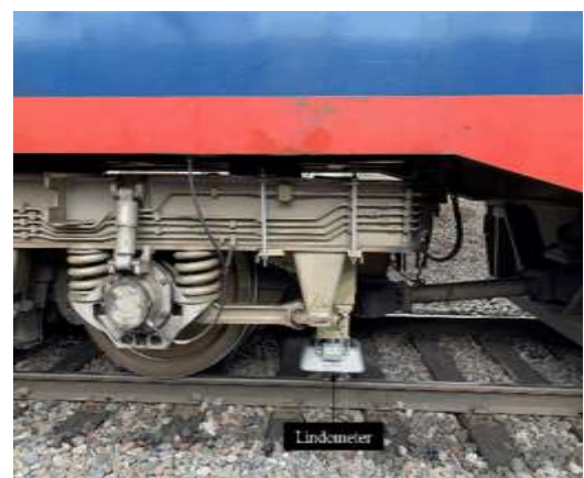
Figure 1 Differential eddy current measurement system (Lindometer) mounted on a freight train
